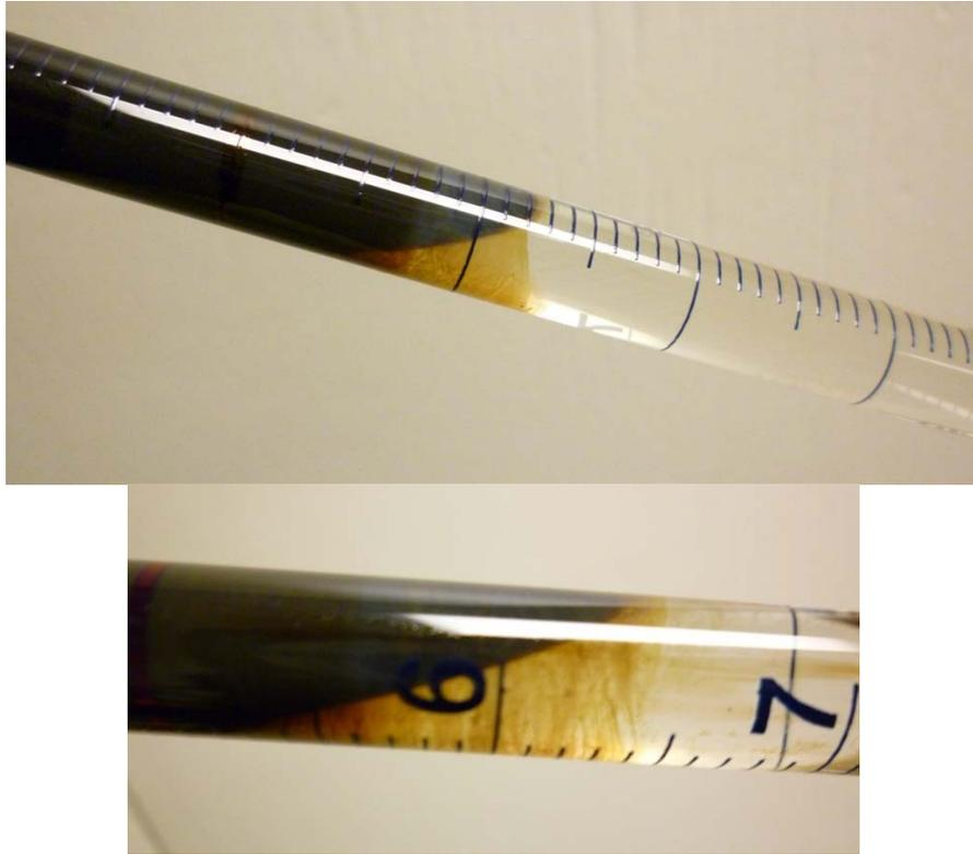
**Figure 3** - Visual examination of type III microemulsion fluidity by tilting and twisting the pipet.
